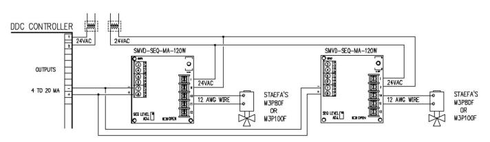
The SMVD-MIS is used for sequencing two valves using isolated 4-20mA inputs. The 4-20mA signal MUST be able to source 1000 Ohms of input resistance. Follow setup instructions on application #5.
