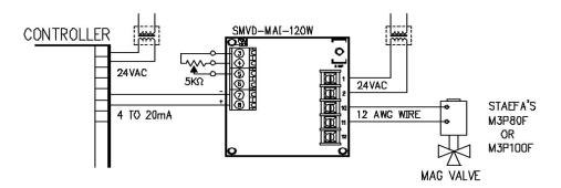
The SMVD-MAI can be used to provide a minimum position or flow. This is done by connecting a 5K Ohm potentiometer from terminals 3 to 4 and the wiper to terminal 5. The SMVD-MAI selects the highest of the two input signals and converts to the phase cut signal.
