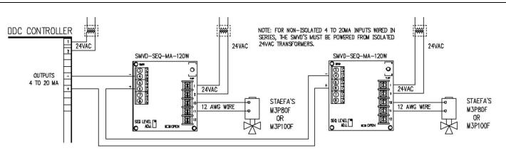
The SMVD-SEQ can be used for sequencing two valves using a 4-20mA input signal. For 1/2 valve operation remove shorting jumper JP1, this doubles the amplifier gain. Manually set your input signal to 50% (1/2 operation) for the 1st valve. Then adjust the 20K Ohm sequencing level pot for 18V phase cut output. Manually set your input signal to 100% for the 2nd valve. Then adjust the 20K Ohm sequencing level pot on the 2nd SMVD for 18V phase cut output.
