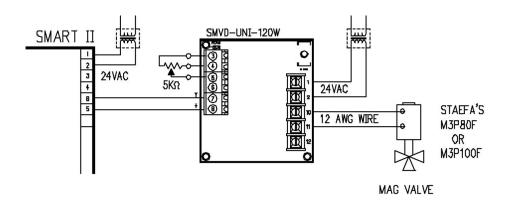
The SMVD-UNI can be used to provide a minimum position or flow. This is done by connecting a 5K Ohm potentiometer from terminals 3 to 4 and the wiper to terminal 5. The SMVD-UNI selects the highest of the two input signals and converts to, or amplifies the phase cut signal.
