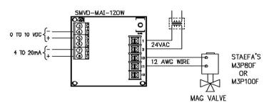
The SMVD-MAI is used for converting 4-20mA, or 0-10VDC signal to 40, 80, or 120 watts to drive the larger STAEFA magnetic valves. The SMVD-MAI-5V is used for converting 4-20mA or 0-5VDC to a phase cut signal JP2 is jumpered for 5 VDC operation otherwise not jumpered for 4-20mA or 10-90% phase cut operation.
