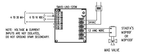
The SMVD-UNI is used for converting 4-20mA, or 0-10VDC or amplifying the 27 watt phase cut signal to 40, 80, or 120 watts to drive the larger STAEFA magnetic valves.
