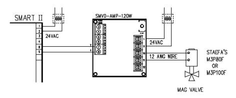
The SMVD-Amp is used for amplifying STAEFA's phase cut signal to drive the larger magnetic valves (40, 80, & 120 watt magnetic valves).
